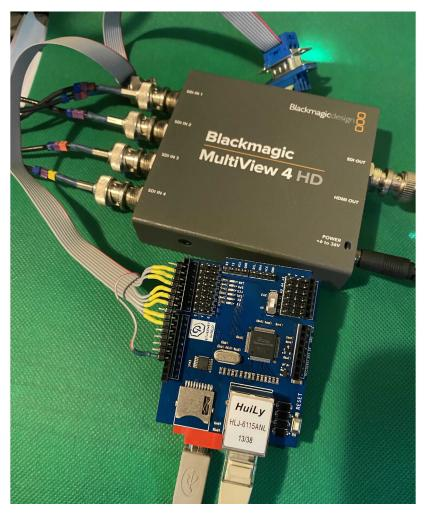
At the bottom is the Arduino Uno and W5100 ethernet shield with a USB connection for power/programming, an ethernet connection and a breakout cable for the control functions. At the top is the 'floating' 9 pin 'D' connector attached to the Blackmagic Multiviewer 4HD.
