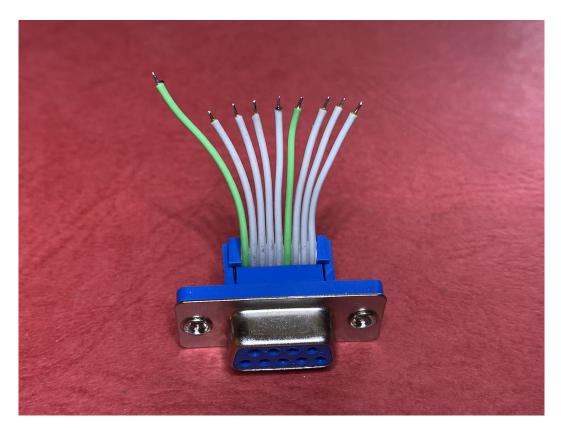
Note the  $\mathbf{1}^{\text{st}}$  cable is connected to pin 1 and is about 8mm longer.
