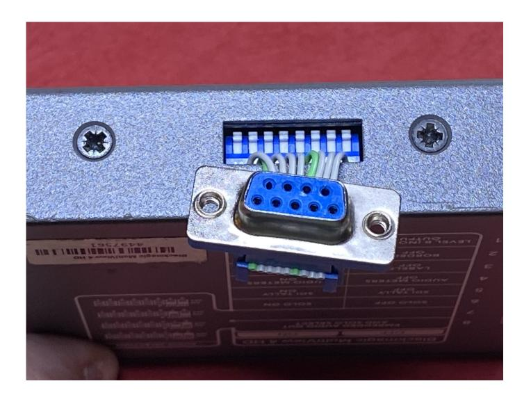
Hopefully you should have retained access to the dip switches for stand alone operation.
