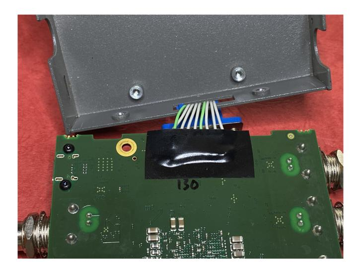
Run some electrical insulation tape across the soldered wires. Note how the ribbon is threaded thru the cover.
