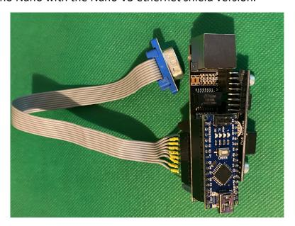
Note that this unit also has a POE (power over ethernet) module attached.
